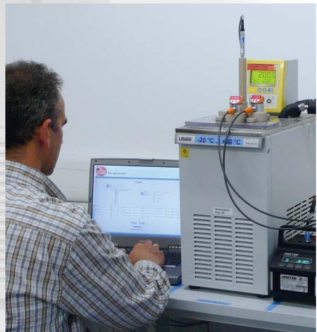
Calibration of temperature sensors
